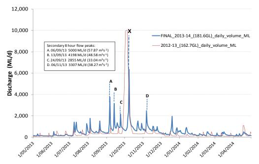
Figure 2. Snowy River below Jindabyne mean daily discharge pattern for 2013/14 (blue), with one primary (X) and four secondary (A,B,C,D) hourly flow peaks (dotted lines) compared with 2012/13 mean daily flow pattern (red).
