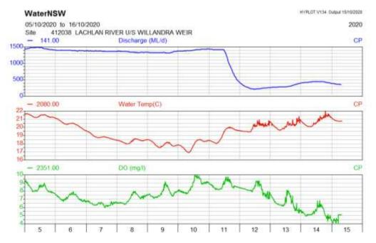
Figure 4: Discharge (ML/day), water temperature (°C) and dissolved oxygen (mg/L) in the Lachlan River at Willandra Weir
