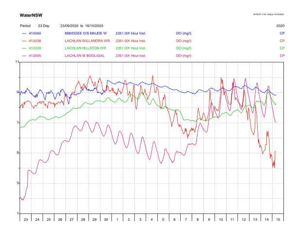
Figure 3: Continuous dissolved oxygen (mg/L) for the Murrumbidgee and Lachlan rivers
