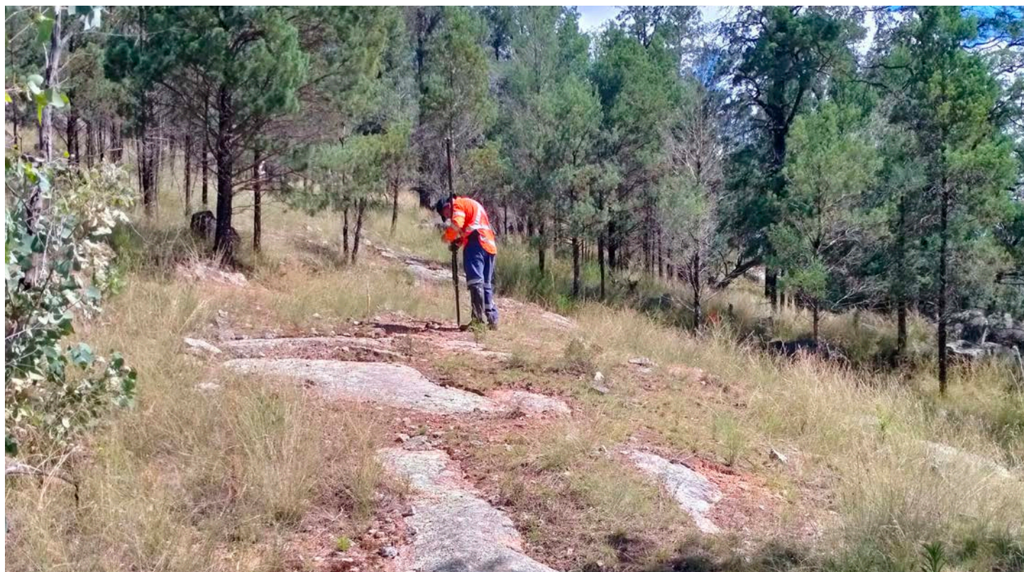
Pictured right and below: Tests of rock and soil help determine suitability for the proposed raised dam wall.
