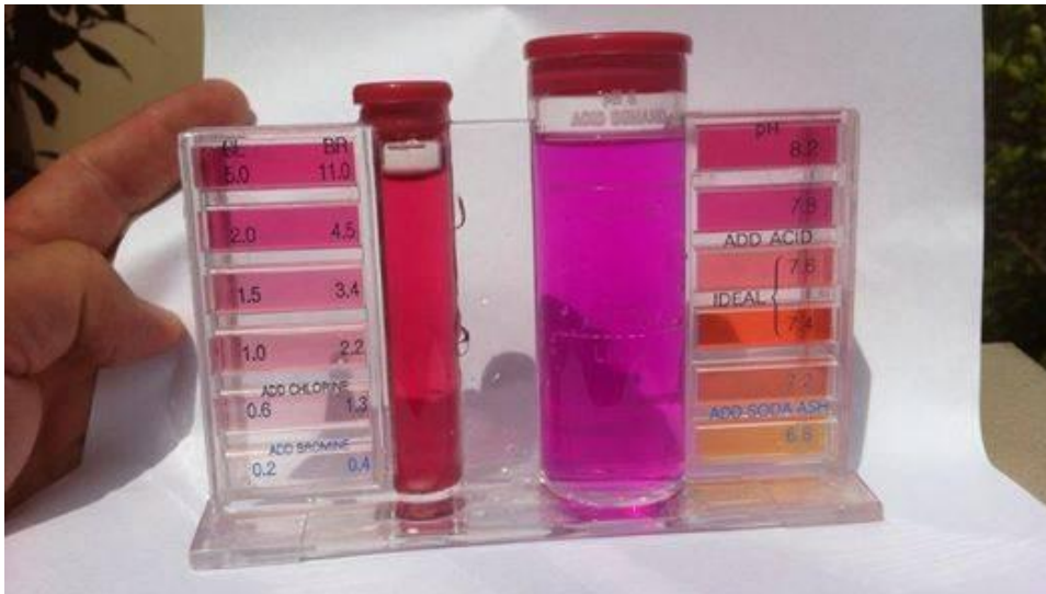
Figure 2. Commercial customer self-testing of the drinking water shows very high levels of chlorine. Gloucester Advocate, 25 March 2015.
