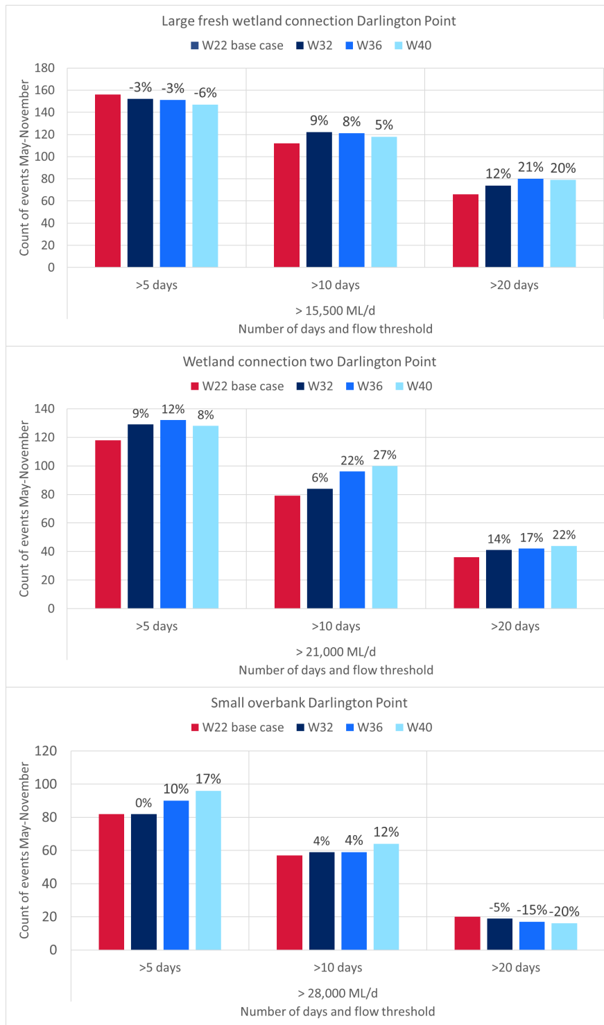
Figure 11: Count of events between May – November at Darlington Point (410021) for more than 5, 10 and 20 days at flow thresholds top: large fresh (wetland connection one, 15,500 ML/d), middle: wetland connection two (21,000 ML/d), bottom: small overbank (28,000 ML/d)
