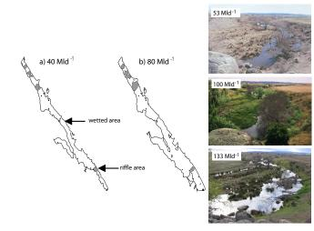
Figure 1 (left): HEC-GeoRAS hydraulic model of Snowy River at Blackburn Creek showing a 50 per cent increase in total wetted area and riffle area at river flows from a) 40 Mld<sup>-1</sup> (mega litres per day) and b) 80 Mld<sup>-1</sup>. Photopoint monitoring of the Snowy River at 53, 100 and 133 Mld<sup>-1</sup>. Source: Rose (in press).
