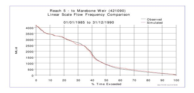
Figure 3.10: Flow Calibration: Results for Reach 5
