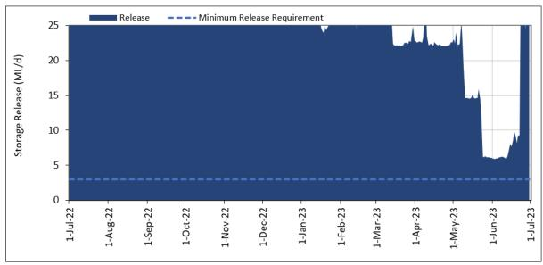
Figure 32 : Chaffey dam releases and minimum release requirements
