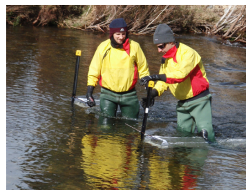
Plate 3. 25x25cm nets with 1.5m tails and 250um mesh arrayed along a transect in the Thredbo River to sample drifting invertebrates and transported CPOM. Nets are fixed to star pickets using 6mm steel roundbar 5 . Photo: D. Coleman ▶
