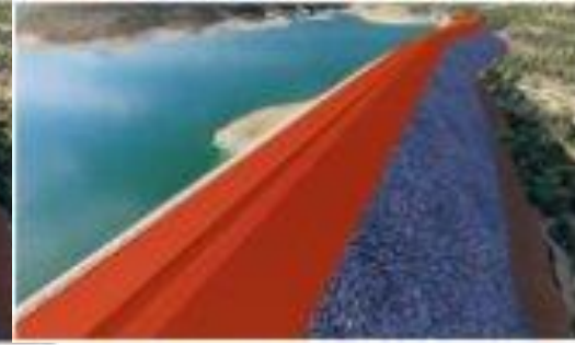
Stage 5 – Finish raising dam wall
